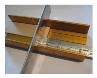
When measuring for the cut be sure to count the thickness of your saw blade if you are measuring the material to be removed.
